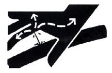
Openings in the skin and minor cuts can be infected from hydraulic fluid. If injured by escaping hydraulic fluid, see a doctor at once. Gangrene can result. Without immediate treatment, serious infection and reactions can occur.
