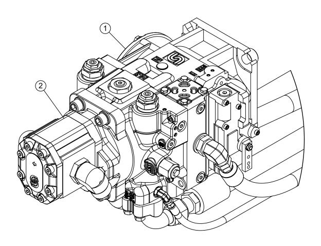
RH PUMPS ARE FOR REPTO OR PTO DRIVE LH PUMPS ARE FOR FEPTO DRIVE
