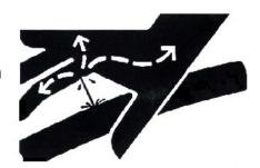
Openings in the skin and minor cuts are susceptible to infection from hydraulic fluid. If injured by escaping hydraulic fluid, see a doctor at once. Gangrene can result. Without immediate treatment, serious infection and reactions can occur.
