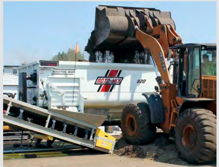
920-18 Stationary Rotary Mixer (920 cu. ft. capacity) Operating on composting site
